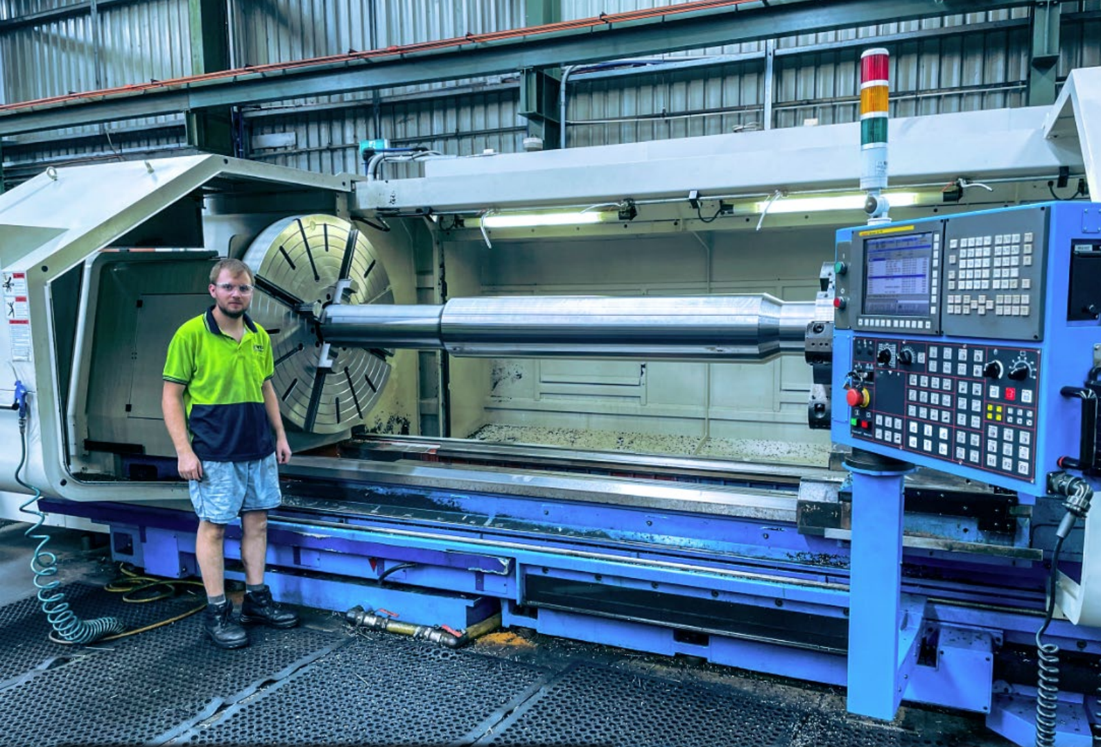
360mm diameter x 2800mm long axle shaft in the AJAX CNC Lathe
